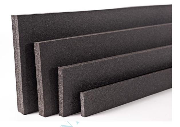
Jointflex is a closed cell, crossed linked, non-absorbent polyethylene expansion joint fillerboard for use in expansion and isolation joints in concrete and masonry structures. Jointflex is nonabsorbent and has excellent properties allowing it to be used in water retaining and excluding structures where potable, salt, chlorine and sewerage water is present.
